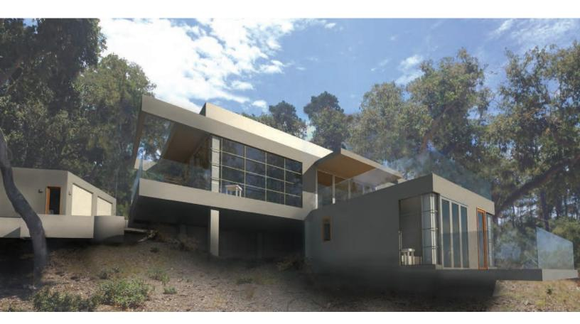
This house is divided into five 20'x20' modules that are organized to fit between the existing trees on site. The modular design will facilitate and simplify the construction process. The exterior of the home and the adjacent garage are clad with gray-brown cement fiber panels that invoke the tone and texture of the surrounding Coast Live Oaks. Folding glass panels open the house up to an additional 2,000 SF of outdoor deck area.
